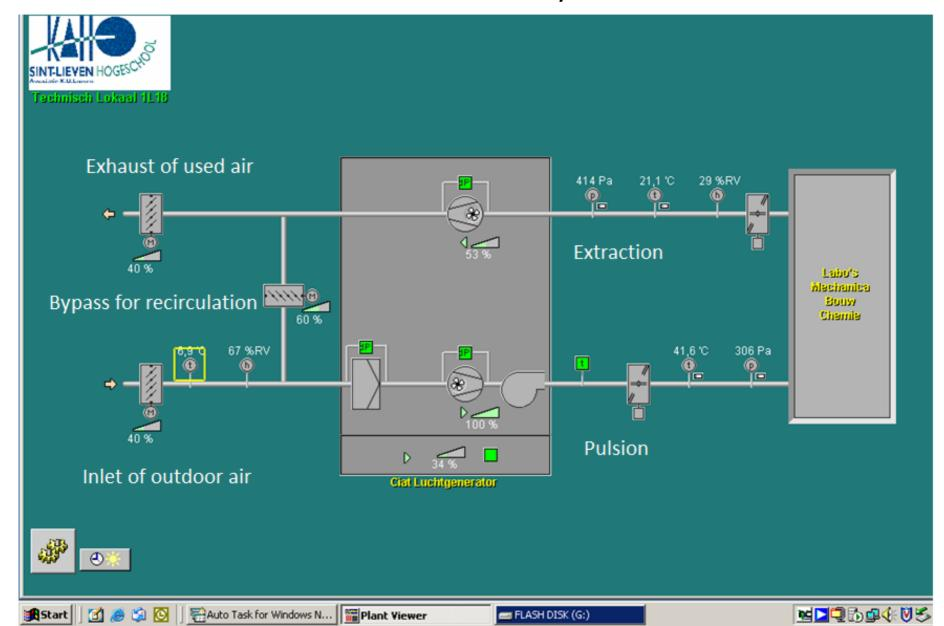
Air mixing centre (plenum): mixes outdoor air with recycled air. The percentage of fresh air is controlled by a motor driven valves.
