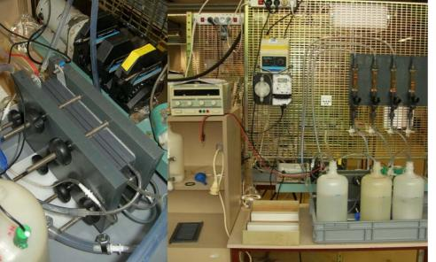
→ Modified Electrodialysis ion exchanger in an electrodialysis stack
