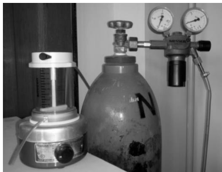
Figure 2. Laboratory apparatus for „dead-end“ ultrafiltration
