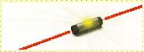
Moreover, the lifetime of graphite tube would be severely reduced if the sample contains high concentrations of certain compounds such as strongly oxidizing acids.
