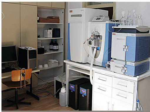
FP7 CEFSER Lab for Mass Spectrometry: Thermo Fisher Scientific UHPLC Accela –Exactive MS (on the left) and Thermo Fisher Scientific UHPLC Accela - TSQ Vantage™ MS/MS (on the right)
