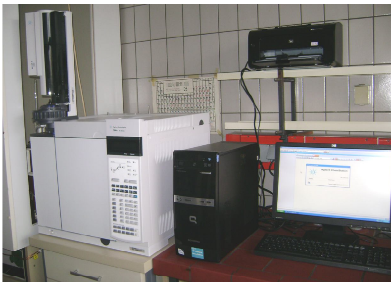
Agilent 7890 GC/ECD system installed at the laboratory of the Faculty of Technology
