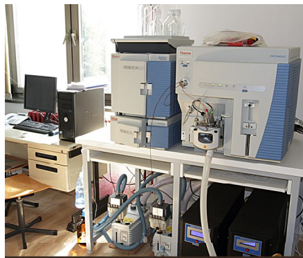
FP7 CEFSER Lab for Mass Spectrometry: Thermo Fisher Scientific UHPLC Accela –Exactive MS (on the left) and Thermo Fisher Scientific UHPLC Accela - TSQ Vantage™ MS/MS (on the right)
